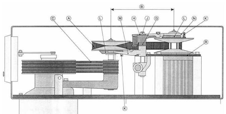
**NEVER** move the base for motor (**R**)(in the oblong holes), this is a factory setting and is **NOT** used to tighten the belts. If the entire unit is to be exchanged, reference the below table. Models W30-W40(P) Distance (B) 11 1/2 inches Models W60-W150 Distance (B) 12 1/4 inches
